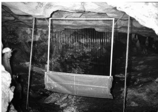
Top. Elery asked Andy and Jan Spate to construct a harp bat trap to assist with research into southern bentwing bats in Bat Cave, Naracoorte. This was Australia's first harp trap built in 1966.
